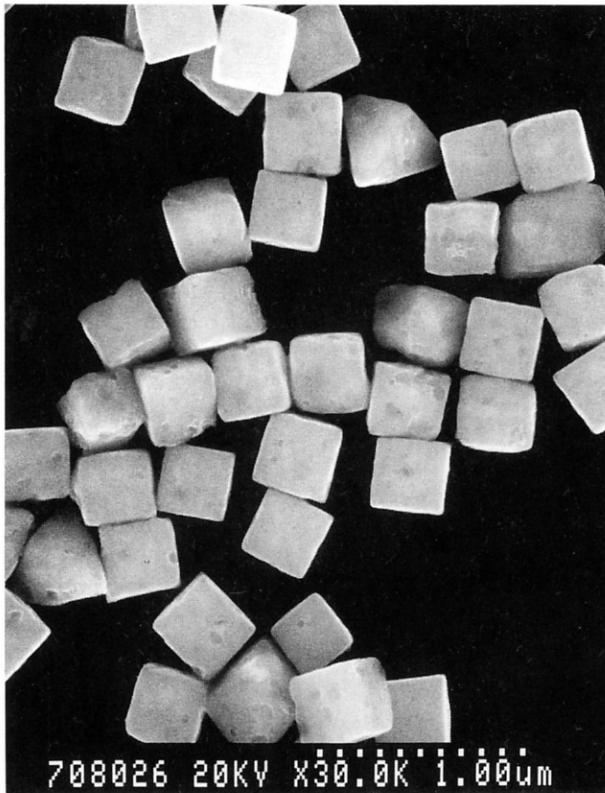
Fig.5 HSG silver halide crystals used in EFM-100E
