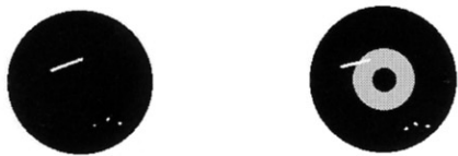
(1) ideal defect image of lens (2) real defect image with ghost
