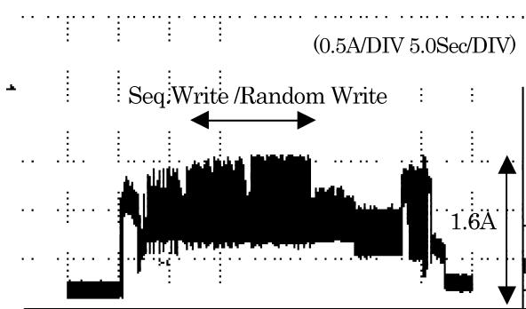
Fig. 4 Current wave at low speed model
