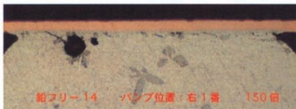
Fig.5 BGA Solder Ball After Thermal Shock Test
