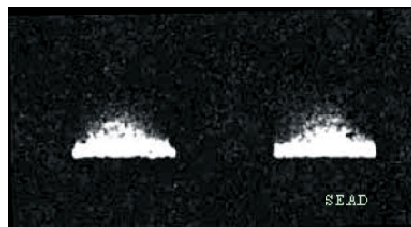
Fig.6 Photograph of light leak of deteriorated shutter
