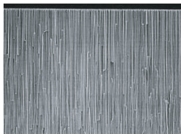
Fig.5 Sectional scanning electron micrograph view of CsBr phosphor
