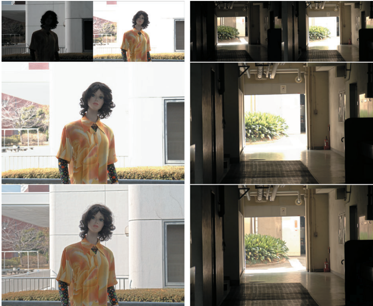
Fig.8 Images obtained through contrast improvement processing. Input images are linear/log images converted from linear high-dynamic range images synthesized from short- and long-exposure time images. Top: short- and long-exposure time images. Middle: images from conventional image data processing of input images. Bottom: images from our contrast improvement
