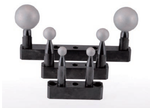
Fig.13 Artifacts for inspection of the RANGE7
