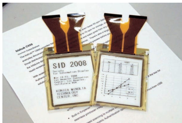
Fig.9 Images of electronic paper (3.5 inch & 113 ppi) with silver electrodeposition driven by LTPS-TFTs
