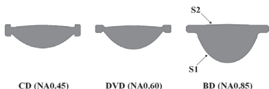
Fig.3 Optical surface shape comparison among objective lenses of differing NA
