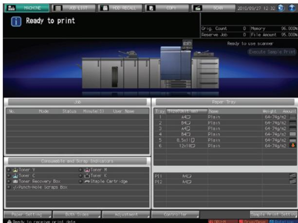
Fig. 5 Screen showing machine status when "Machine" icon is clicked.
