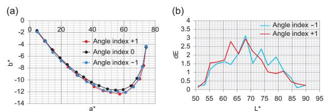
Figure 7 (a) indicates  $a^*$  and  $b^*$  variations between 0% to 100% dot percent of Magenta under different skew angle. (b) shows lightness( $L^*$ ) vs color difference( $dE$ ). color difference at angle index +1 and -1 are calculated between angle index 0 and each angle index.
