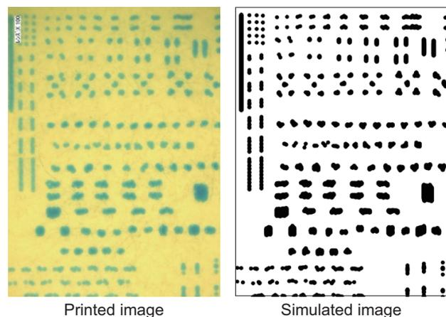
Figure 4 Comparison between a printed image and the estimated image.
