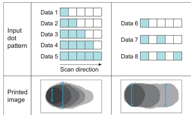
Figure 3 Example of obtaining the parameter for dot pattern simulation. Line width and line length change depending on variable input data patterns.
