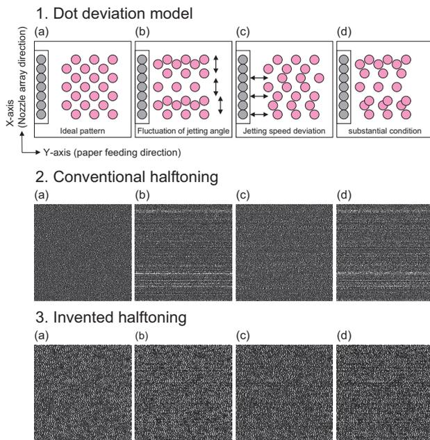
Figure 5 Simulated example of dot patterns under dot position's deviation.
