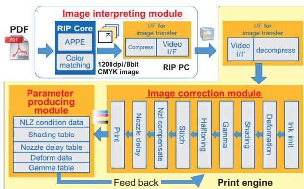
Figure 2 Outline of the image correction data flow.
