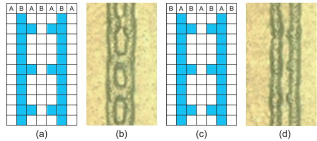
Figure 6 Differences of coverage depending on a differences of dot placement order. (a) (c) indicate input images and (b), (d) indicate printed results. Data for column A is printed before data for column B is printed.
