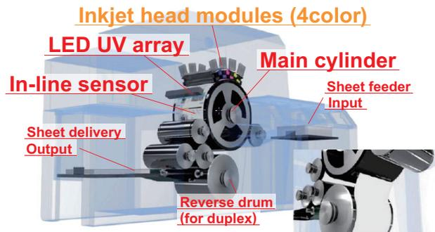
Figure 1 Structural illustration of AquarioJet KM-1 system.
