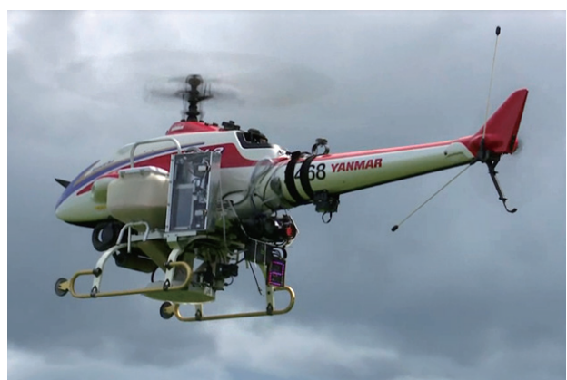
Fig. 12 A GPS-equipped, unmanned helicopter applies fertilizer selectively as guided by a fertilizer map.
