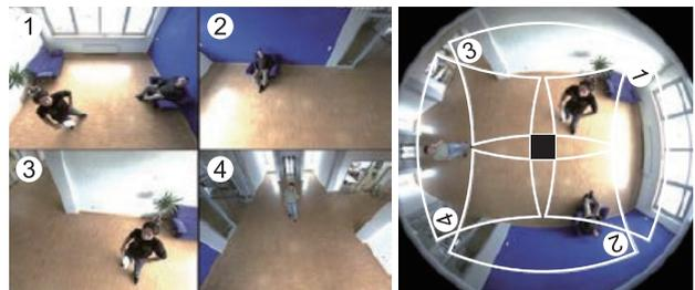
Fig. 9 Four virtual pan-tilt-zoom (PTZ) camera views are derived from a single 360 deg hemispheric camera.
