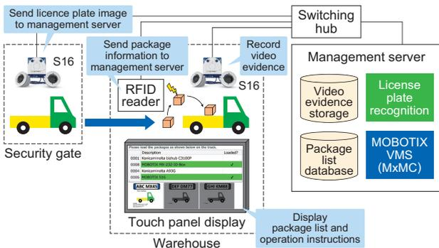
Fig. 7 Demo system configuration.
