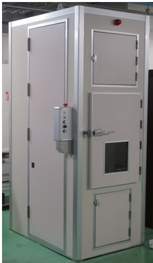
Fig. 5 Outer appearance of prototype non-destructive inspection system.
