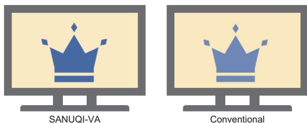
Fig. 4 SANUQI has a refractive index closer to that of PVA than conventional material, and optical loss is accordingly smaller, thereby increasing contrast. This figure shows images having a contrast difference of 10%.
