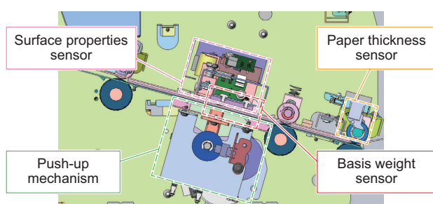
Fig. 12 Layout of inline-type optical basis weight sensor, paper thickness sensor, and surface property sensor for PP machine. The paper type and basis weight of the fed paper are determined with the three types of sensors disposed on the conveyance path.
