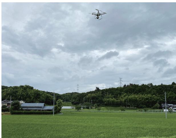
Fig. 5 Remote sensing by drone equipped with multi-spectral camera.
