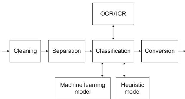
Fig. 11 Digitization process diagram.
