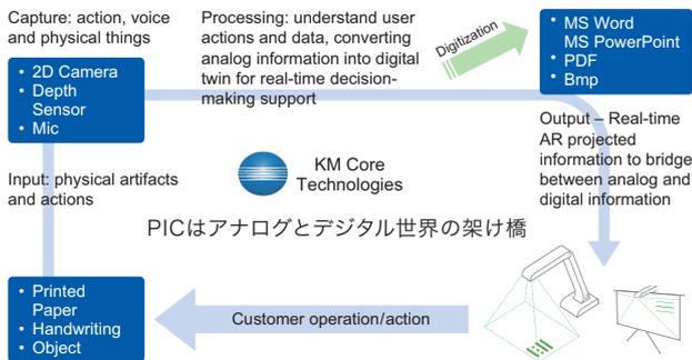
Fig. 1 High level concept of PIC.
