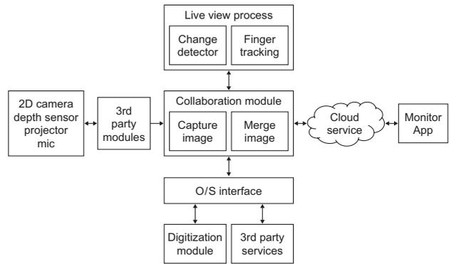
Fig. 3 High level PIC block diagram.
