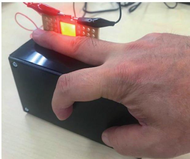
Fig. 9 An example of side illumination for finger vein authentication.
